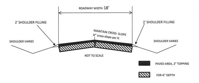
FDR WILL BE 18FT AND 6" DEPTH. MAINTAIN PROPER CROSS SLOPE FOR DRAINAGE. RESURFACE FULL WIDTH WITH 220LBS PER SQUARE YARD RECYCLED ASPHALTIC CONCRETE 12.5MM SUPERPAVE, GP 2 ONLY, INCL BITUM MATL & H LIME .
