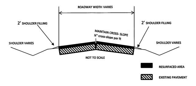
RETAIN EXISTING PAVEMENT AND MAINTAIN PROPER CROSS SLOPE. PATCHING AND LEVEL 85 LBS PER SQUARE YARD OR AS DIRECTED BY ENGINEER. RESURFACE FULL WIDTH WITH 135 LBS PER SQUARE YARD RECYCLED ASPHALTIC CONCRETE 9.5MM SUPERPAVE, GP 2 ONLY, INCL BITUM MATL & H LIME.
