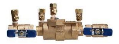
The DCA is the most common type of approved backflow prevention device for use in underground or in-line installations. In-line (or below-grade) simply means that the backflow device is parallel with the piping of the sprinkler system; unlike the PVB, the DCA does not have to be installed 12 inches above the highest point in the system. Some areas do require above-ground installation, so check with local authorities before installing below ground.
